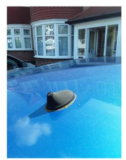
Desirable: Electrical / Controls > In Car Entertainment Systems > Aerial / Antenna > Missing
