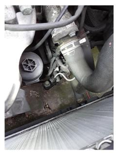
Essential: Transmission > Hydraulic System > Clutch Slave Cylinder > Evidence of Fluid Leaks, clean and investigate cause
