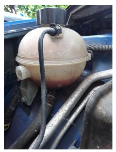
Essential: Engine Compartment > Coolant Level > Coolant Content > Below Minimum, top up system, replenish lost antifreeze and pressure to identify possible leaks
