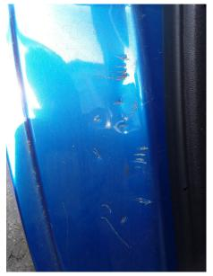
Desirable: Interior / Luggage Compartment > Interior Sills / Shut Area > Right Rear Interior Sill / Shut > Dents and corrosion evident, recommend remedial attention to prevent further deterioration
