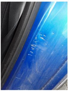
Desirable: Interior / Luggage Compartment > Interior Sills / Shut Area > Left Rear Interior Sill / Shut > Dents and corrosion evident, recommend remedial attention to prevent further deterioration
