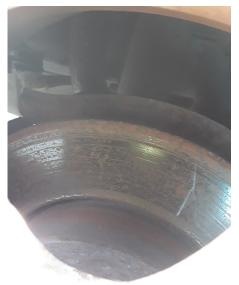
Essential: Brake System > Discs / Pads / Linings > Both Front Brake Discs > Corroded Brake Discs > Corroded and ridged
