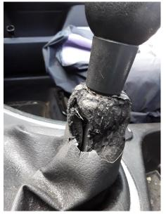
Desirable: Interior / Luggage Compartment > Dash Panel {Condition} > Gear Lever Gaiter > Perished and split
